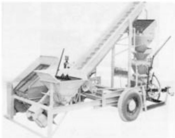
Figure 5: Proportioning, mixing, predampening mixer.
