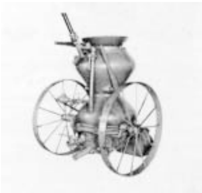
Figure 1: Double chamber gun (Allentown).
