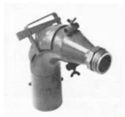
Figure 13: Casting head used in gun-casting.
